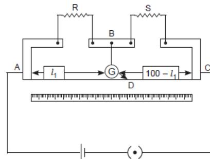
In a meter bridge, the point D is a neutral point (figure).
