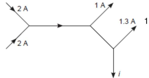
The figure below shows currents in a part of electric circuit. The current  $i$  is \_\_\_\_\_.
