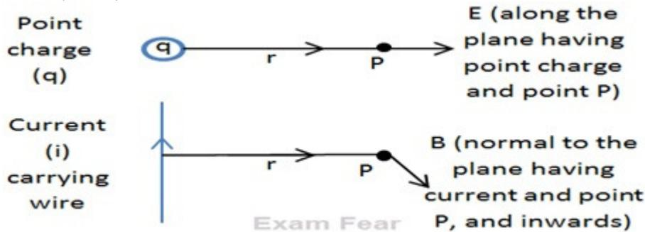
The first diagram shows the electric field (E) due to a point charge (q)
