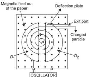
(i) The machine is cyclotron. A cyclotron is in
