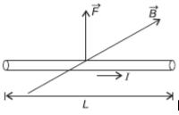
Magnetic field will act in the direction perpendicular to the direction of flow of current.
