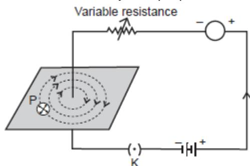
**Magnetic field around a straight conducting wire.**
