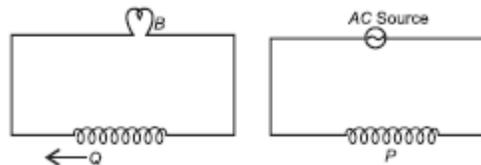
ANS: (a) The bulb B lights because an emf is induced in coil Q due to change in magnetic flux crossing through it.
