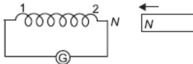
**Justification:** Lenz's law complies with the principle of conservation of energy. For example, when the N-pole of a bar magnet is pushed into a coil as shown, the direction of induced current in the coil will be such that the end 2 of the coil will act as N-pole. Thus, work has to be done against the magnetic repulsive force to push the magnet into the coil. The electrical energy produced in the coil is at the expense of this work done.
